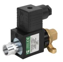
Spartan solenoid valve, 2-way, 2-position, N.C., low lead brass body, 1/4in female NPT inlet(s), 1/4in female NPT outlet(s), Cv=0.24, 200 psi maximum operating pressure, 24 VDC operating voltage, 18mm DIN style wiring plug.
