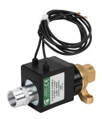
Spartan solenoid valve, 2-way, 2-position, N.C., low lead brass body, 1/4in female NPT inlet(s), 1/4in female NPT outlet(s), Cv=0.24, 200 psi maximum operating pressure, 24 VDC operating voltage, 18in 22 AWG pigtail.
