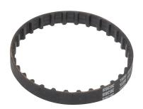
SureMotion timing belt, 1/5in XL pitch, 1/4in wide, 30 tooth, 6in pitch length (circumference), neoprene, fiberglass reinforced.
