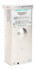
Bryant manual motor controller, enclosed, 60A, 600 VAC, 3-pole, 30hp, wall mount, die-cast aluminum housing, NEMA 3R, UL 508 rated.
