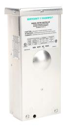
Bryant manual motor controller, enclosed, 60A, 600 VAC, 2-pole, 20hp, wall mount, die-cast aluminum housing, NEMA 3R, UL 508 rated.
