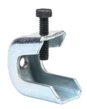
Minerallac screw-on beam clamp, 200 lbs. Package of 25. For use with flanges up to 3/4in and 3/8-16 threaded rod.
