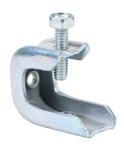
Minerallac screw-on beam clamp, 75 lbs. Package of 50. For use with flanges up to 1/2in and 1/4-20 threaded rod.
