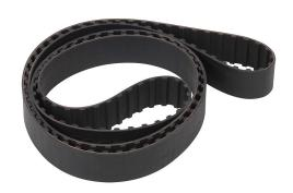
SureMotion timing belt, 3/8in L pitch, 1in wide, 160 tooth, 60in pitch length (circumference), neoprene, fiberglass reinforced.
