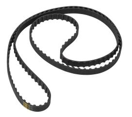
SureMotion timing belt, 3/8in L pitch, 1/2in wide, 160 tooth, 60in pitch length (circumference), neoprene, fiberglass reinforced.
