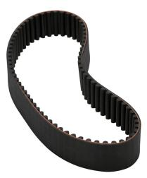
SureMotion timing belt, 8mm 8M pitch, 30mm wide, 75 tooth, 600mm pitch length (circumference), neoprene, fiberglass reinforced.
