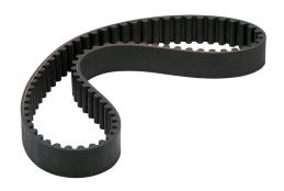
SureMotion timing belt, 8mm 8M pitch, 20mm wide, 75 tooth, 600mm pitch length (circumference), neoprene, fiberglass reinforced.
