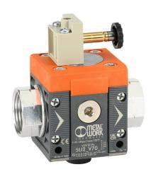
Metal Work shut-off valve, 3-port (3-way), 2-position, single solenoid spring return, N.C., 1in female NPT inlet(s), 1in female NPT outlet(s), G1/4 female BSPP exhaust(s), Cv=4.4. For use with Syntesi Size 2 air prep components.
