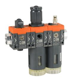
Metal Work Syntesi Size 2 pneumatic combination unit, valve-filter-regulator-lubricator, 1in female NPT inlet(s), 1in female NPT outlet(s), 0 to 120 psig range, clear technopolymer bowl, manual/semi-automatic drain, manual shutoff valve.
