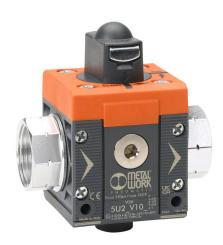
Metal Work shut-off valve, 3-port (3-way), 2-position, twist, N.C., 1in female NPT inlet(s), 1in female NPT outlet(s), G1/4 female BSPP exhaust(s), Cv=4.4. For use with Syntesi Size 2 air prep components.
