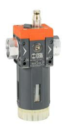
Metal Work Syntesi Size 2 pneumatic lubricator, 1in female NPT inlet(s), 1in female NPT outlet(s), clear technopolymer bowl, bowl guard.
