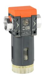
Metal Work Syntesi Size 2 pneumatic filter, particulate and moisture separation, 1in female NPT inlet(s), 1in female NPT outlet(s), manual/semi-automatic drain, clear technopolymer bowl, bowl guard.
