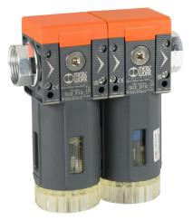
Metal Work Syntesi Size 2 pneumatic combination unit, filtercoalescing filter, 1in female NPT inlet(s), 1in female NPT outlet(s), clear technopolymer bowl, manual/semi-automatic drain.
