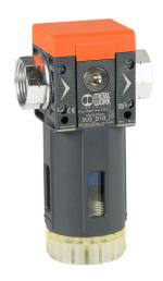
Metal Work Syntesi Size 2 pneumatic filter, coalescing oil removal, 1in female NPT inlet(s), 1in female NPT outlet(s), manual/semiautomatic drain, clear technopolymer bowl, bowl guard.
