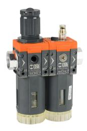
Metal Work Syntesi Size 2 pneumatic combination unit, filter-regulator-lubricator, 1in female NPT inlet(s), 1in female NPT outlet(s), 0 to 120 psig range, clear technopolymer bowl, manual/semi-automatic drain.
