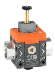
Metal Work soft start valve, 3-port (3-way), 2-position, single solenoid spring return, N.C., 1in female NPT inlet(s), 1in female NPT outlet(s), G1/4 female BSPP exhaust(s), Cv=5.3. For use with Syntesi Size 2 air prep components.
