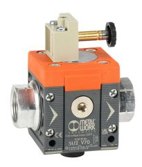
Metal Work shut-off valve, 3-port (3-way), 2-position, single solenoid spring return, N.C., 3/4in female NPT inlet(s), 3/4in female NPT outlet(s), G1/4 female BSPP exhaust(s), Cv=4.4. For use with Syntesi Size 2 air prep components.
