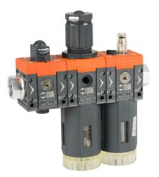
Metal Work Syntesi Size 2 pneumatic combination unit, valvefilter-regulator-lubricator, 3/4in female NPT inlet(s), 3/4in female NPT outlet(s), 0 to 120 psig range, clear technopolymer bowl, manual/semi-automatic drain, manual shutoff valve.
