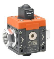
Metal Work shut-off valve, 3-port (3-way), 2-position, twist, N.C., 3/4in female NPT inlet(s), 3/4in female NPT outlet(s), G1/4 female BSPP exhaust(s), Cv=4.4. For use with Syntesi Size 2 air prep components.
