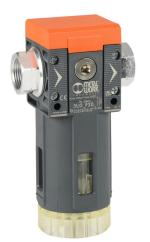
Metal Work Syntesi Size 2 pneumatic filter, particulate and moisture separation, 3/4in female NPT inlet(s), 3/4in female NPT outlet(s), manual/semi-automatic drain, clear technopolymer bowl, bowl guard.
