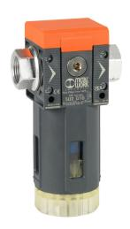
Metal Work Syntesi Size 2 pneumatic filter, coalescing oil removal, 3/4in female NPT inlet(s), 3/4in female NPT outlet(s), manual/semi-automatic drain, clear technopolymer bowl, bowl guard.
