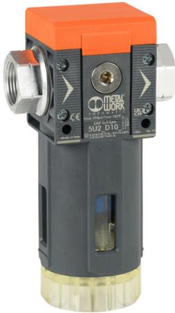
Metal Work Syntesi Size 2 pneumatic filter, coalescing oil removal, 3/4in female NPT inlet(s), 3/4in female NPT outlet(s), manual/semi-automatic drain, clear technopolymer bowl, bowl guard.
