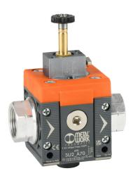
Metal Work soft start valve, 3-port (3-way), 2-position, single solenoid spring return, N.C., 3/4in female NPT inlet(s), 3/4in female NPT outlet(s), G1/4 female BSPP exhaust(s), Cv=5.3. For use with Syntesi Size 2 air prep components.
