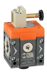
Metal Work shut-off valve, 3-port (3-way), 2-position, single solenoid spring return, N.C., 1/2in female NPT inlet(s), 1/2in female NPT outlet(s), G1/4 female BSPP exhaust(s), Cv=4.4. For use with Syntesi Size 2 air prep components.
