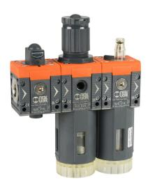
Metal Work Syntesi Size 2 pneumatic combination unit, valve-filter-regulator-lubricator, 1/2in female NPT inlet(s), 1/2in female NPT outlet(s), 0 to 120 psig range, clear technopolymer bowl, manual/semi-automatic drain, manual shutoff valve.
