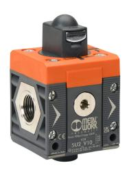
Metal Work shut-off valve, 3-port (3-way), 2-position, twist, N.C., 1/2in female NPT inlet(s), 1/2in female NPT outlet(s), G1/4 female BSPP exhaust(s), Cv=4.4. For use with Syntesi Size 2 air prep components.
