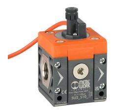
Metal Work pressure switch, air, 1/2in female NPT process connection, 7.5 to 145 psi set point, N.O./N.C. complementary, 2m 3-wire cable. For use with Syntesi Size 2 air prep components.
