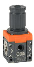
Metal Work Syntesi Size 2 pneumatic regulator, 1/2in female NPT inlet(s), 1/2in female NPT outlet(s), 0 to 120 psig range.
