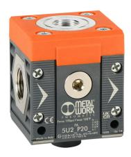
Metal Work air distribution block, 1/2in female NPT inlet(s), (1) 1/4in female NPT, (1) 3/8in female NPT and (1) 1/2in female NPT outlet(s). For use with Syntesi Size 2 air prep components.
