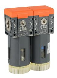
Metal Work Syntesi Size 2 pneumatic combination unit, filter-coalescing filter, 1/2in female NPT inlet(s), 1/2in female NPT outlet(s), clear technopolymer bowl, manual/semi-automatic drain.
