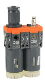
Metal Work Syntesi Size 2 pneumatic combination unit, filter-regulator-lubricator, 1/2in female NPT inlet(s), 1/2in female NPT outlet(s), 0 to 120 psig range, clear technopolymer bowl, manual/semi-automatic drain.
