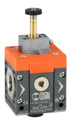
Metal Work soft start valve, 3-port (3-way), 2-position, single solenoid spring return, N.C., 1/2in female NPT inlet(s), 1/2in female NPT outlet(s), G1/4 female BSPP exhaust(s), Cv=5.3. For use with Syntesi Size 2 air prep components.
