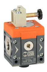
Metal Work shut-off valve, 3-port (3-way), 2-position, single solenoid spring return, N.C., 3/8in female NPT inlet(s), 3/8in female NPT outlet(s), G1/4 female BSPP exhaust(s), Cv=4.1. For use with Syntesi Size 2 air prep components.
