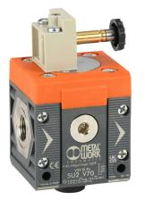
Metal Work shut-off valve, 3-port (3-way), 2-position, single solenoid spring return, N.C., 3/8in female NPT inlet(s), 3/8in female NPT outlet(s), G1/4 female BSPP exhaust(s), Cv=4.1. For use with Syntesi Size 2 air prep components.
