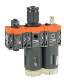
Metal Work Syntesi Size 2 pneumatic combination unit, valve-filter-regulator-lubricator, 3/8in female NPT inlet(s), 3/8in female NPT outlet(s), 0 to 120 psig range, clear technopolymer bowl, manual/semi-automatic drain, manual shutoff valve.
