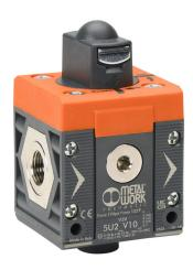
Metal Work shut-off valve, 3-port (3-way), 2-position, twist, N.C., 3/8in female NPT inlet(s), 3/8in female NPT outlet(s), G1/4 female BSPP exhaust(s), Cv=4.1. For use with Syntesi Size 2 air prep components.
