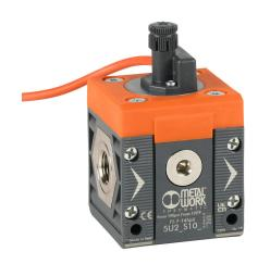
Metal Work pressure switch, air, 3/8in female NPT process connection, 7.5 to 145 psi set point, N.O./N.C. complementary, 2m 3-wire cable. For use with Syntesi Size 2 air prep components.
