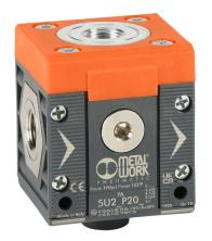
Metal Work air distribution block, 3/8in female NPT inlet(s), (1) 1/4in female NPT and (2) 3/8in female NPT outlet(s). For use with Syntesi Size 2 air prep components.
