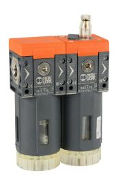
Metal Work Syntesi Size 2 pneumatic combination unit, filter-lubricator, 3/8in female NPT inlet(s), 3/8in female NPT outlet(s), clear technopolymer bowl, manual/semi-automatic drain.
