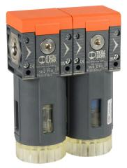
Metal Work Syntesi Size 2 pneumatic combination unit, filtercoalescing filter, 3/8in female NPT inlet(s), 3/8in female NPT outlet(s), clear technopolymer bowl, manual/semi-automatic drain.
