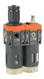
Metal Work Syntesi Size 2 pneumatic combination unit, filter-regulator-lubricator, 3/8in female NPT inlet(s), 3/8in female NPT outlet(s), 0 to 120 psig range, clear technopolymer bowl, manual/semi-automatic drain.
