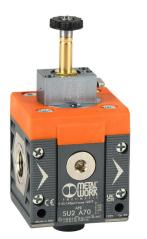
Metal Work soft start valve, 3-port (3-way), 2-position, single solenoid spring return, N.C., 3/8in female NPT inlet(s), 3/8in female NPT outlet(s), G1/4 female BSPP exhaust(s), Cv=4.1. For use with Syntesi Size 2 air prep components.
