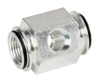
Metal Work air distribution block, 1/2in female NPT inlet(s), (1) 1/2in female NPT and (2) 3/8in female NPT outlet(s). For use with Syntesi Size 2 air prep components.
