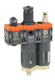
Metal Work Syntesi Size 1 pneumatic combination unit, valve-filter-regulator-lubricator, 3/8in female NPT inlet(s), 3/8in female NPT outlet(s), 0 to 120 psig range, clear technopolymer bowl, manual/semi-automatic drain, manual shutoff valve.
