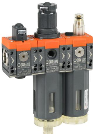
Metal Work Syntesi Size 1 pneumatic combination unit, valve-filter-regulator-lubricator, 3/8in female NPT inlet(s), 3/8in female NPT outlet(s), 0 to 120 psig range, clear technopolymer bowl, manual/semi-automatic drain, manual shutoff valve.
