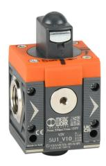
Metal Work shut-off valve, 3-port (3-way), 2-position, twist, N.C., 3/8in female NPT inlet(s), 3/8in female NPT outlet(s), G1/8 female BSPP exhaust(s), Cv=1.6. For use with Syntesi Size 1 air prep components.
