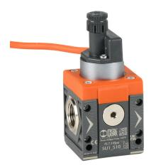
Metal Work pressure switch, air, 3/8in female NPT process connection, 7.5 to 145 psi set point, N.O./N.C. complementary, 2m 3-wire cable. For use with Syntesi Size 1 air prep components.
