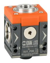
Metal Work air distribution block, 3/8in female NPT inlet(s), (1) 1/8in female NPT, (1) 1/4in female NPT and (1) 3/8in female NPT outlet(s). For use with Syntesi Size 1 air prep components.
