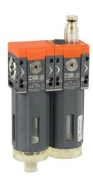
Metal Work Syntesi Size 1 pneumatic combination unit, filter-lubricator, 3/8in female NPT inlet(s), 3/8in female NPT outlet(s), clear technopolymer bowl, manual/semi-automatic drain.
